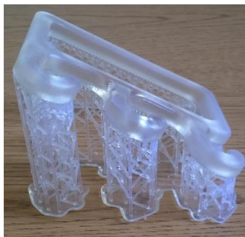
**Figure 10: Build orientation of the SLA part**
