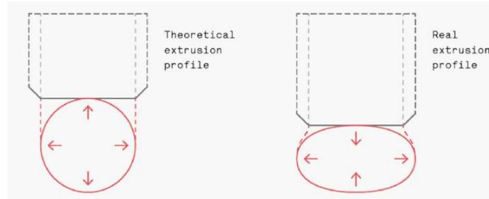
**Figure 12: FFF material extrusion profiles [12]**
