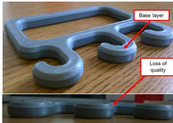
**Figure 6: FFF part defect (base side facing up)**
