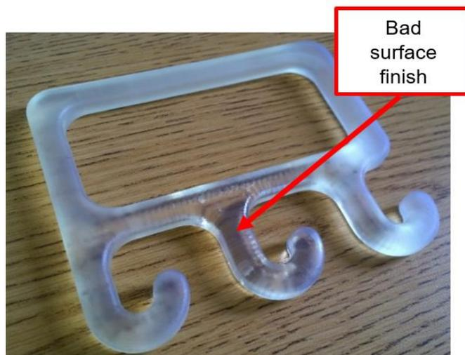
**Figure 9: Bad surface finish defect on the SLA part**
