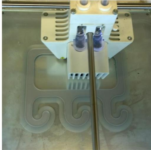
**Figure 8: Horizontal build orientation of the FFF part**
