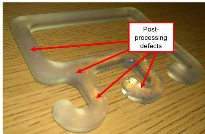
**Figure 11: Defects induced by post-processing**
