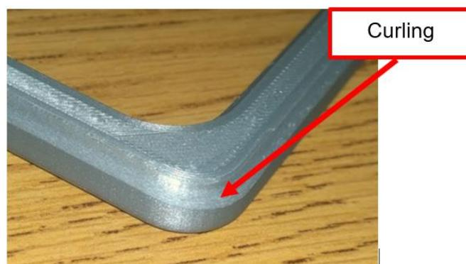
**Figure 7: Curling defect at the corner of the FFF part**
