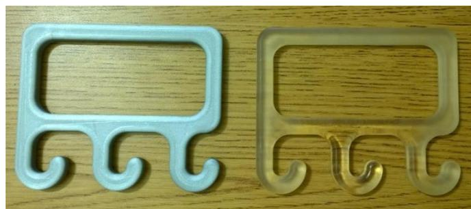
**Figure 2: Finished FFF part (left) and SLA part (right)**
