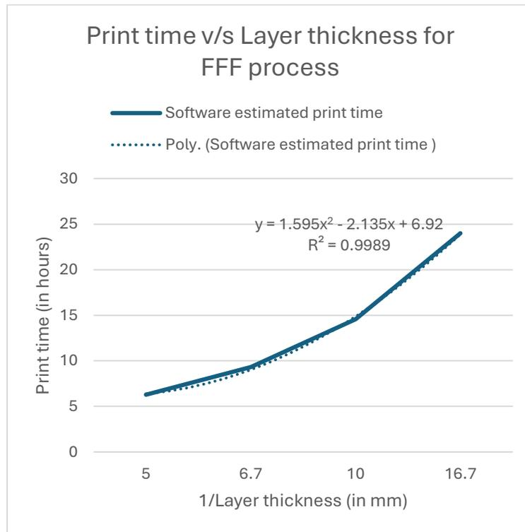
**Figure 14: Regression model of FFF process**
